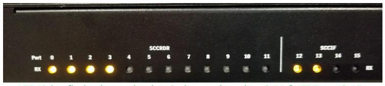
LED Lights flash when radar data is detected on chan 0-11 & IFDT on 12-15
